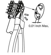
STEP 3: The tips of the wires should be no more than 0.01 inch.
