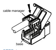
STEP 4: Install cable manager on base. Be sure they snap together completely.
