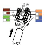
STEP 2: Insert wire pairs into the correct positions (T568A/568B).
